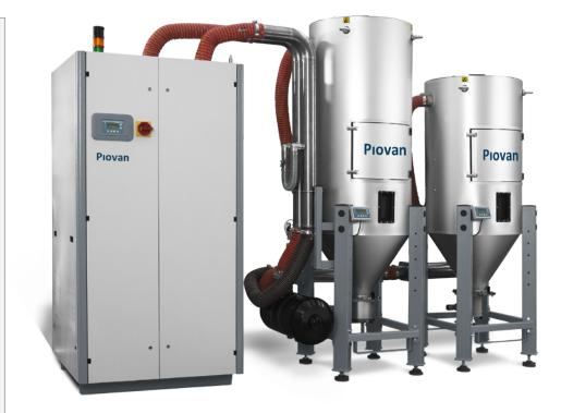
Double desiccant tower models, with an airflow rate from 200 to 800 m³/h, supply air at a dew point lower than -55°C. The process air temperature can be set up to 150°C (200°C for the HT version). The DP 619 - DP 624 Dryer
